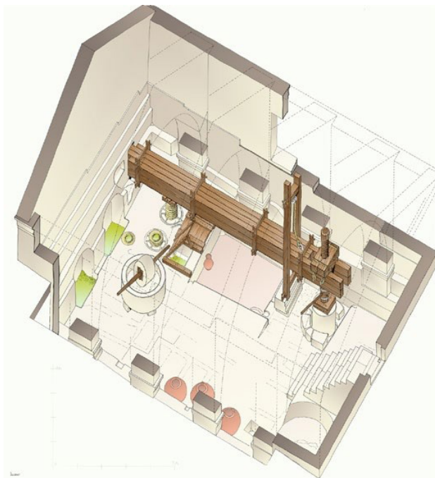
Fig. 9. Reconstruction of the large dual-purpose presses found at Sergilla (Abdulkarim and Charpentier, 2016: 397, Fig. 6)
